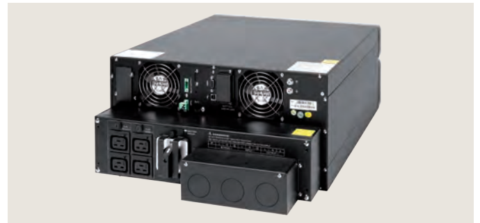
Protect D. 10000 – rear view: flexible, removable connection unit with manual bypass and integrated IEC output distribution with automated locking mechanism
